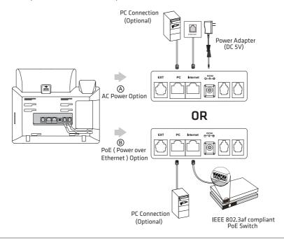
**Note:** If power is provided over Ethernet (PoE) do not connect the power adapter. Make sure the Ethernet cable and switch are PoE-compliant. The phone can also share the network with another network device such as a PC (personal computer). It is an optional connection. **Important!** Do not unplug or remove power to the phone while it is updating firmware and configurations.
